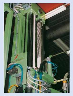
Siegling Proposition timing belts in the vertical axis of an industrial robot.
