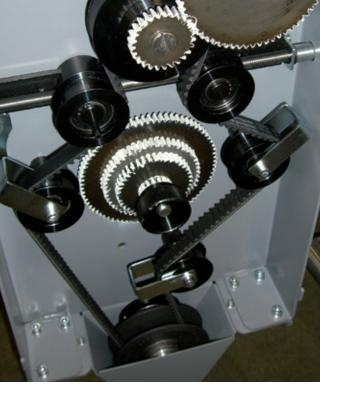
Timing belts in different designs and sections are used in the textile industry. Whether it be small chloroprene timing belts used for spindle drives in texturing machines or high power timing belts in large sections used for main drives right up to polyurethane timing belts, e.g. metre goods welded in circular knitting machines.
