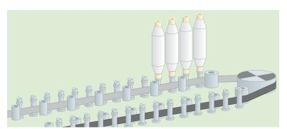
Whether used as power transmission belts for cards and draw frames, or as tangential belts for ring spinning frames and twisters: with the new, reinforced tension members made of polyester or aramide, power requirements are much lower than in belts with conventionally designed tension members.
