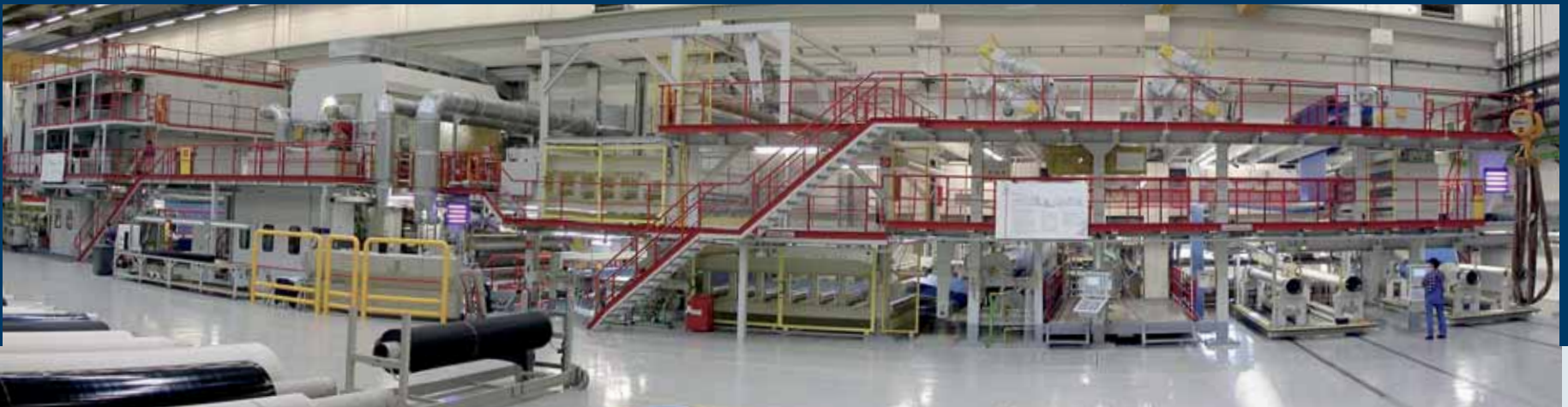
The production machine in the Hanover plant (Germany). The world's biggest four-roll calender for producing conveyor and processing belts.
