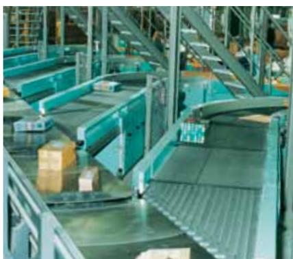
In **merges** the belts that operate in a set, are usually tensioned in one go. This requires particularly low length tolerances. High friction coefficients on the top face guarantee precise transfer to the sorter.
