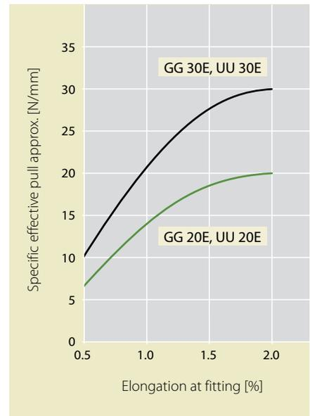
Live roller drives specific effective pull as a function of elongation at fitting
