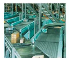
In **merges** the belts that operate in a set, are usually tensioned in one go. This requires particularly low length tolerances.
