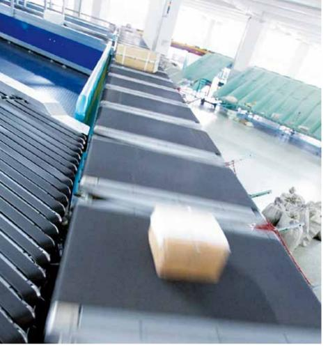
In **cross belt sorters** high acceleration means extremely high friction coefficients in the belt's top face.
