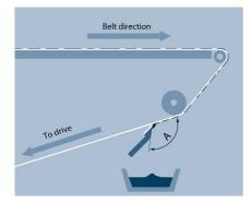
Scraper should lightly touch the belt on the return side just after product has been discharged. The angle "A" normally will be between 100 and 120 degrees.
