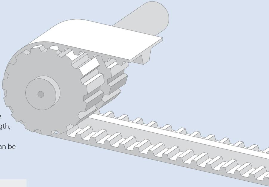
**Timing belts with longitudinal tracking profiles**
