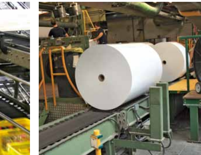
Siegling Transtex can easily handle punctual loads of 1500 kg without damaging the layers of paper on the outside.
