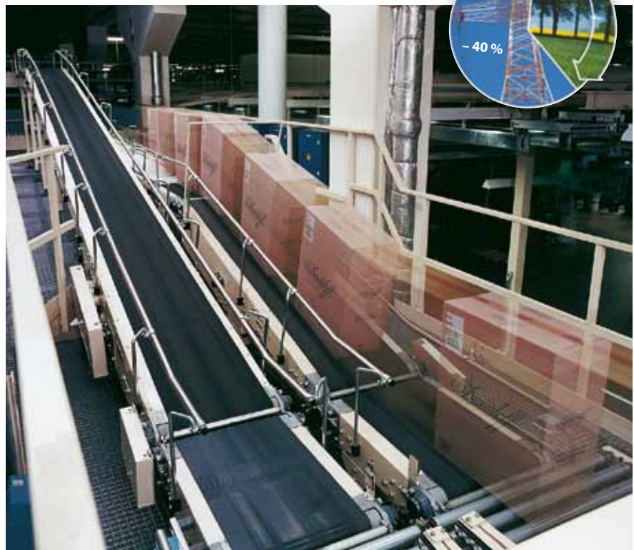
Rapid acceleration in stop-and-go operation with extreme punctual loads place high demands on the belts used.
