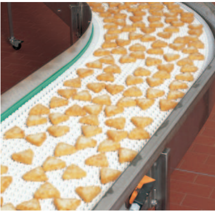
Siegling Prolink curved belts are ideal for space-saving drying or freezing.
