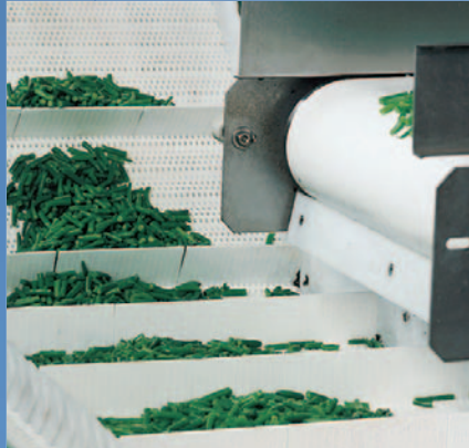
Beans drain through open modules while being conveyed to the next processing step.
