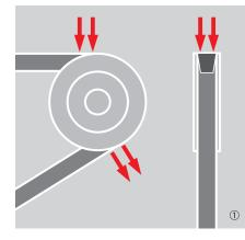
Friction on the sides at the top and bottom, internal friction losses due to hysteresis.
