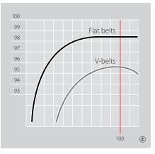
Efficiency of a flat belt (top), efficiency of a V-belt (bottom). Siegling Extremultus flat belts have an efficiency of 98.6 %.
