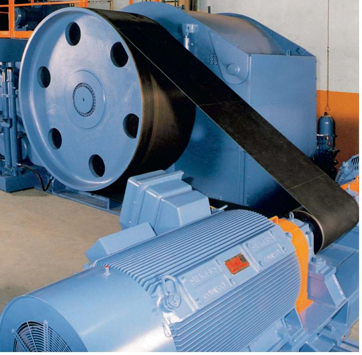
Chipper (wood manufacture), belt type GT 80 P black, width = 1000 mm, P = 1850 kW, v = 65 m/s
